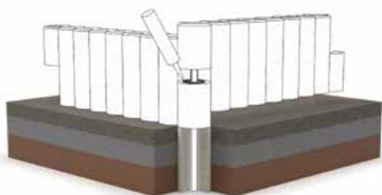
Positioning the chain element with the aid of extended mounting tubes on loose substrate. Glueing of the elements is necessary,
