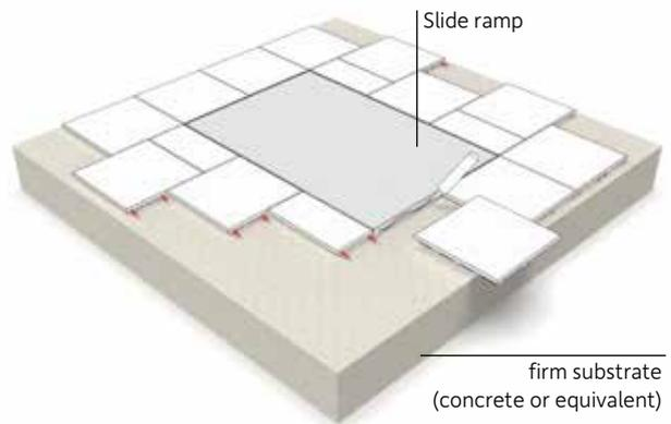
Integration of the slide ramp into the half-board of the Terrasoft Slab 45
